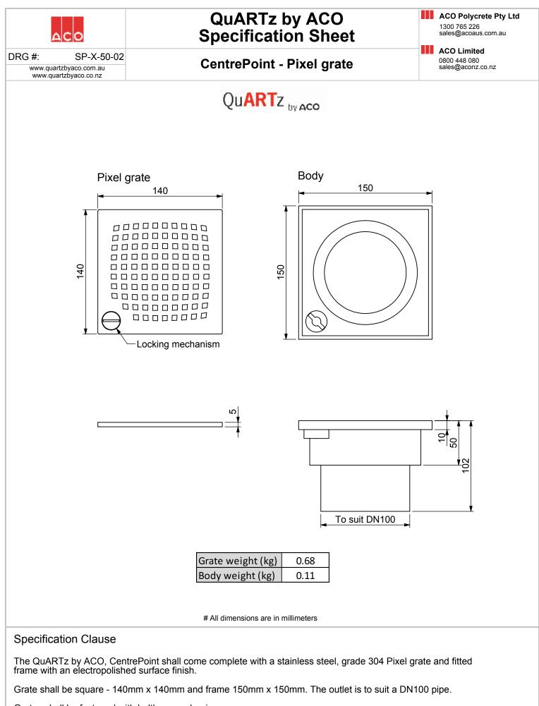
Grates shall be fastened with boltless mechanisms.
