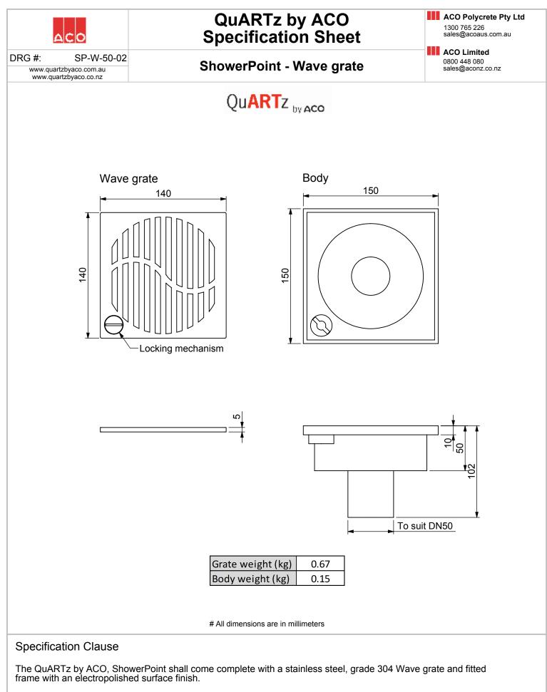
Grate shall be square - 140mm x 140mm and frame 150mm x 150mm. The outlet is to suit a DN50 pipe.
